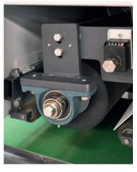
Oscillating edge rounding disc head
