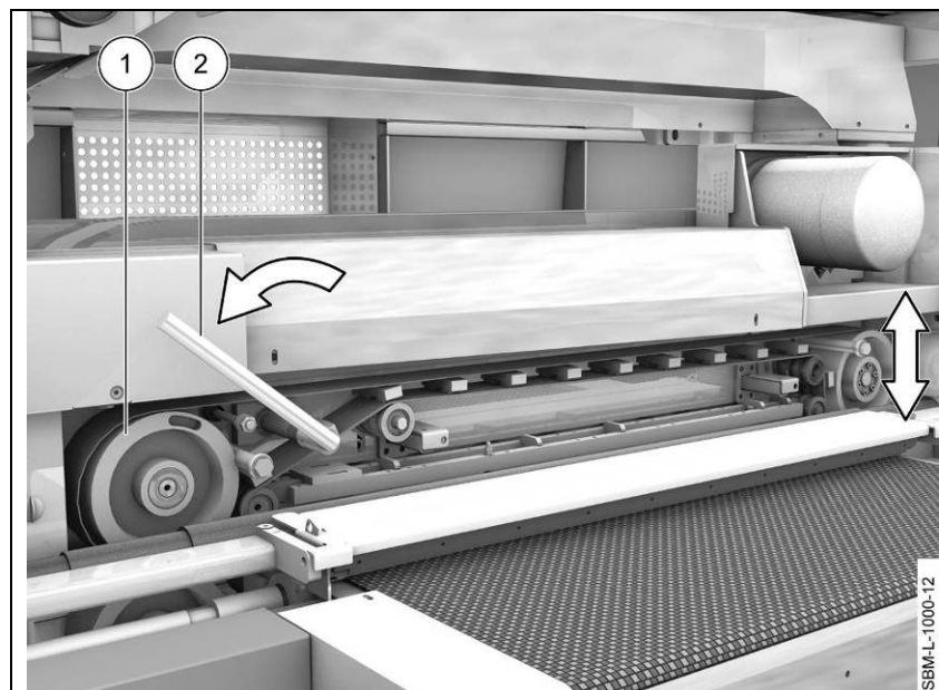
Abb. 41: Changing the grinding belt of the upper G unit
